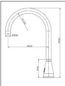
Non-contact self-closing DN 15 Washtable-tap, stainless steel satin; with rotating and lockable curved spout, aerator\*, optosensor.
